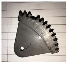
the passenger side seat. As you can see it has seen better days, and was not holding the seat up correctly.
